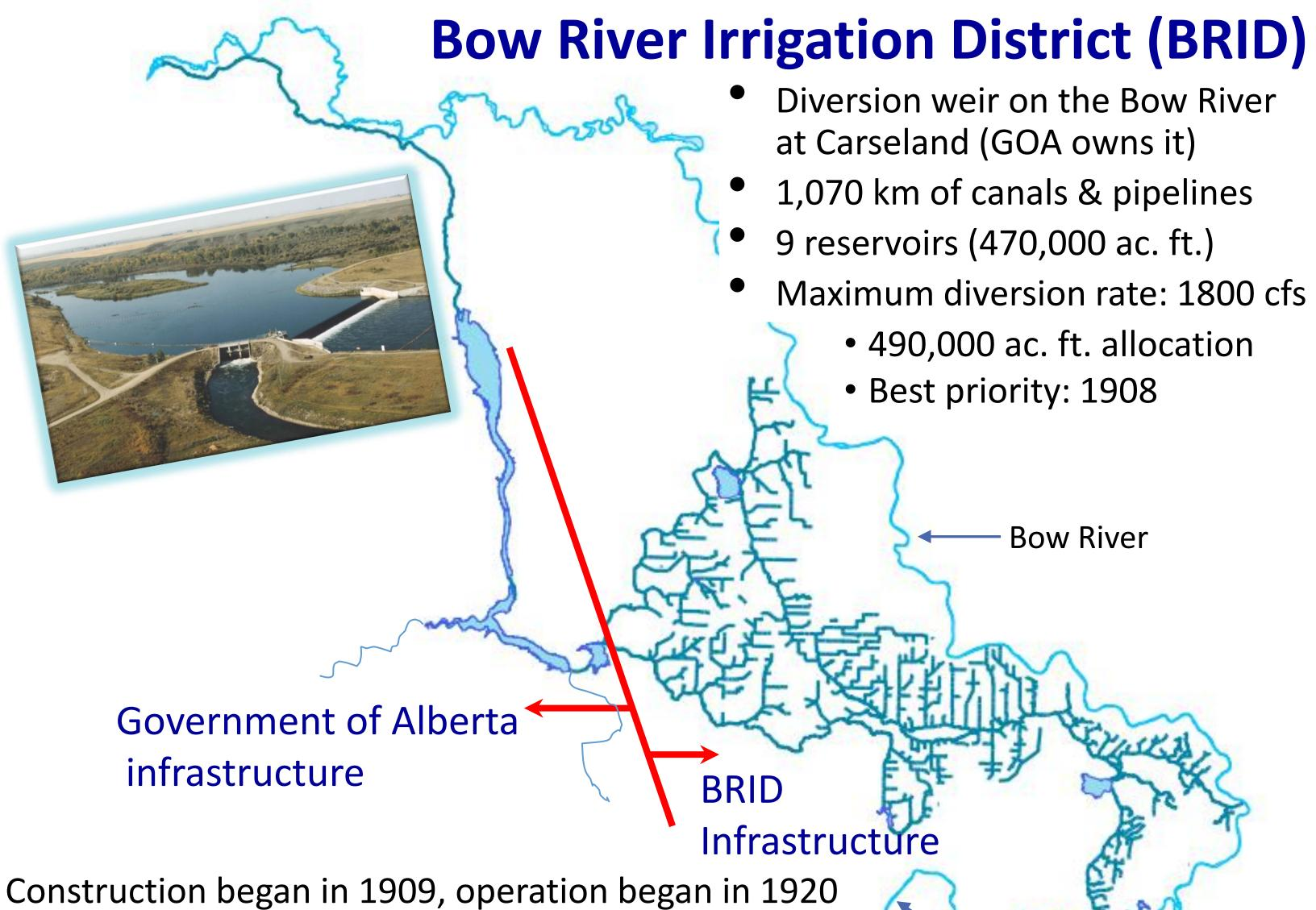
Diversion weir on the Bow River at Carseland (GOA owns it) 1,070 km of canals & pipelines 9 reservoirs (470,000 ac. ft.) Maximum diversion rate: 1800 cfs • 490,000 ac. ft. allocation • Best priority: 1908
